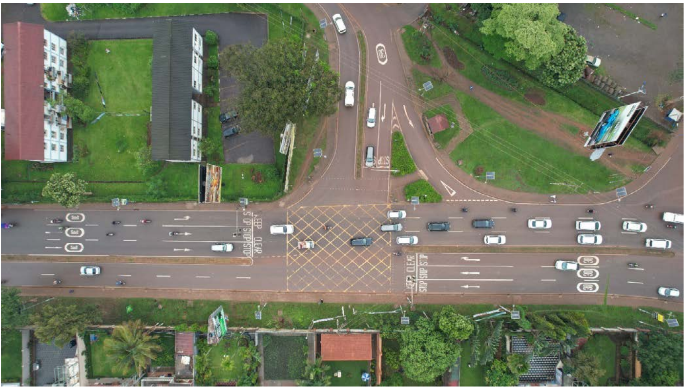
Figure 7.13: Marking of Lane lines, lane direction, speed limit, stop lines and Keep clear at Kira Road- Old Kira Road intersection. Source: WRI
