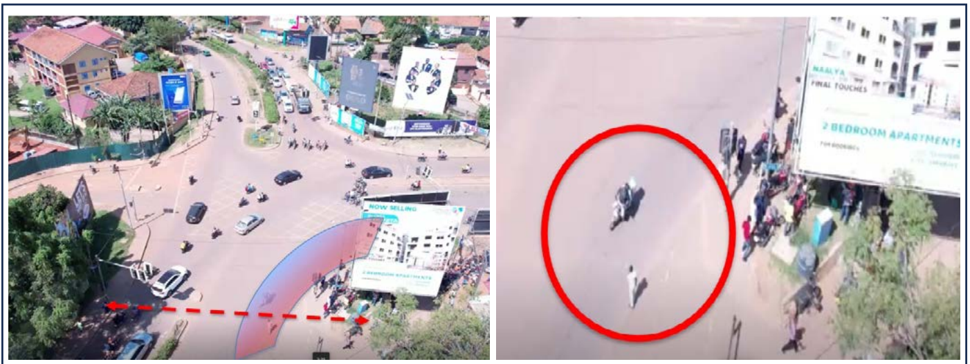
Figure 7.8: Wide slip lane, large turning radius and resulting conflict at Kira Road- Lugogo Bypass intersection
