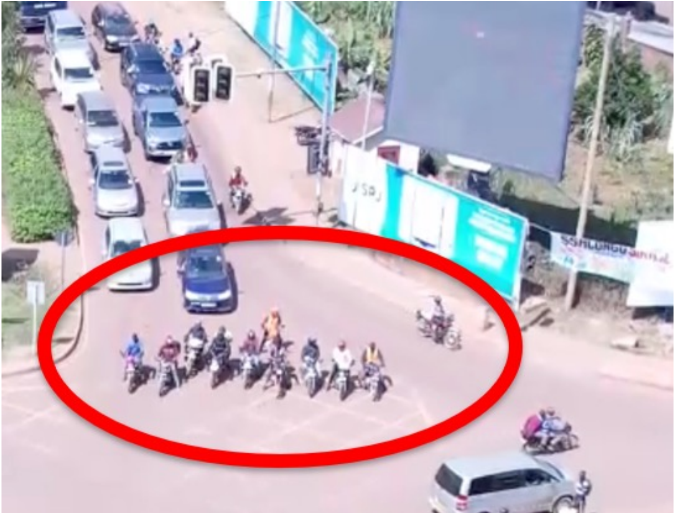
Figure 7.10 : Informal advanced stop box created by motorcycles at the Kira Road- Lugogo Bypass intersection
