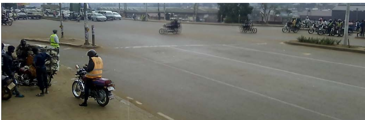
Figure 4.18: Kabuusu intersection, 1.5km from Kitebi primary school (Designated crossing not very visible, no traffic island at crossing point)
