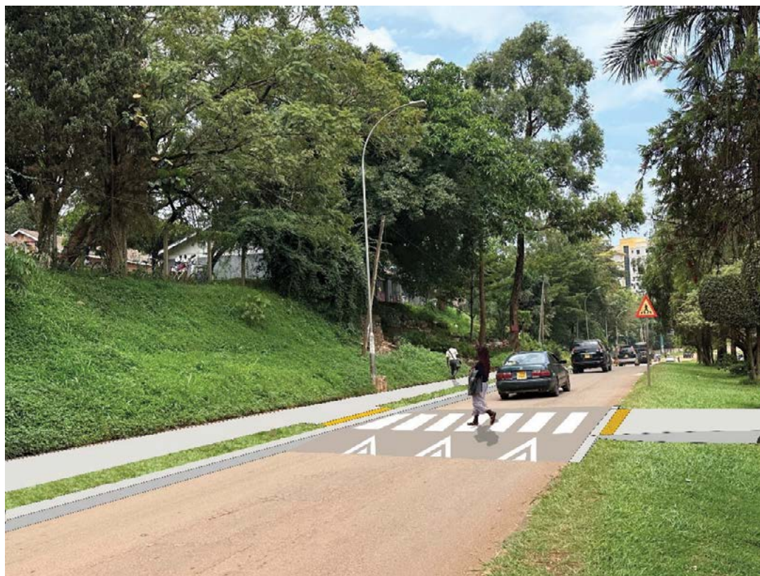
Figure 5.1: Top- October 2023 state of Lugogo bypass near Kololo Senior secondary school; Bottom- Rendering of the same location with introduction of road diet- expansion of the sidewalk into one lane of the road and a raised crossing extended through the median. Credit: Siba El- Samra/WRI
